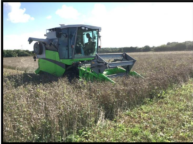
Figure 4. The 2 metre plot combine gives a yield output and samples can be taken in the cab.
