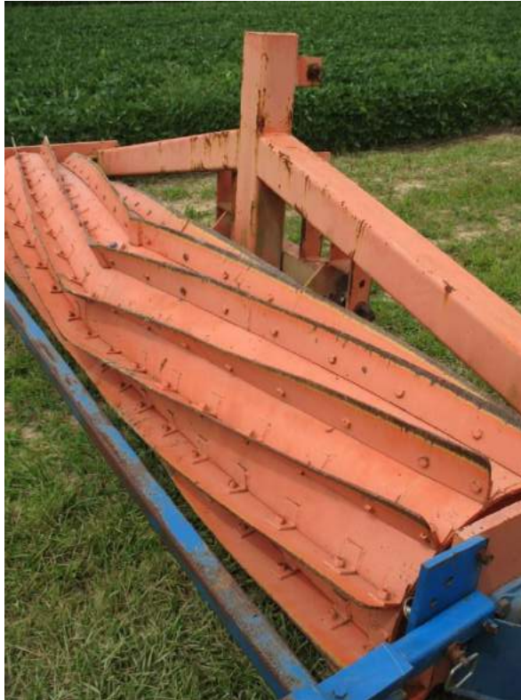
Figure 19: PSU 'crimper roller' used on the cover crop trials
