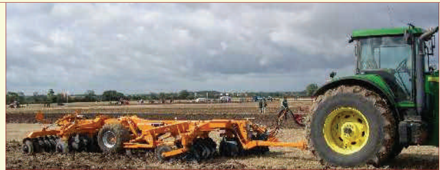
Simba solo heavy disk and packer - shallow non-inversion tillage
