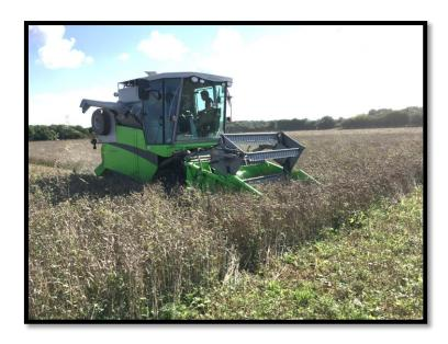
Figure 4. The 2 metre plot combine gives a yield output and samples can be taken in the cab.
