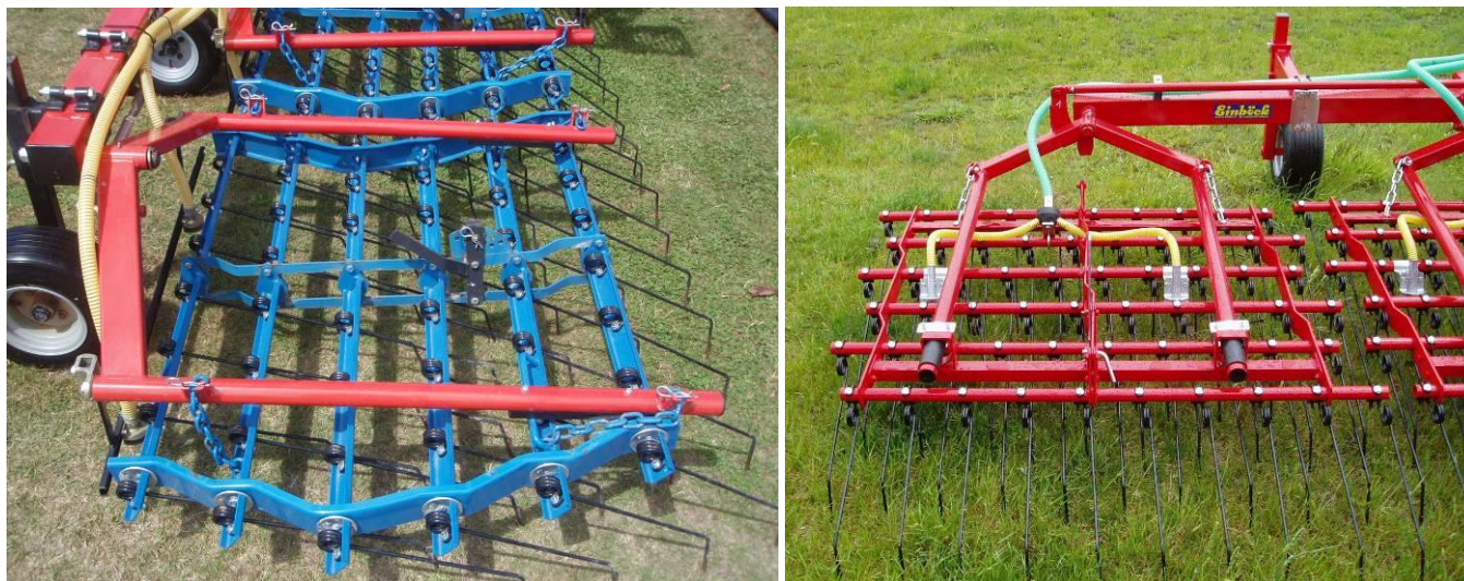
Figure 9. Spring tine weeders - detail of frames and tines
