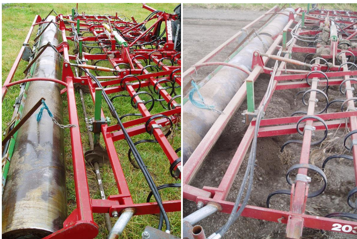
Figure 15. Roller rod-weeder (left), in operation (right). Design and photos copyright © Steam Weeding Ltd. 2015.
