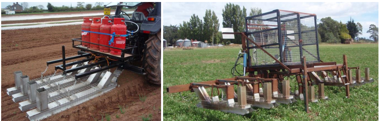
Figure 17. Row flamers, single bed (left) and multi-bed (right). Design and photos copyright © Steam Weeding Ltd. 2015.
