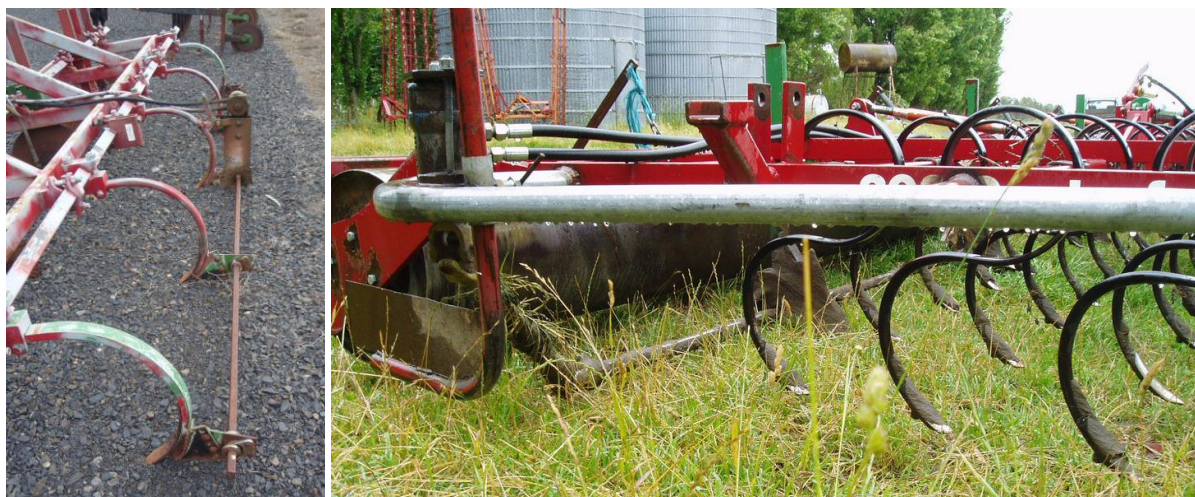
Figure 14. American rod weeder (left), rod weeder built into spring tine cultivator (right). Design and photos copyright © Steam Weeding Ltd. 2015.
