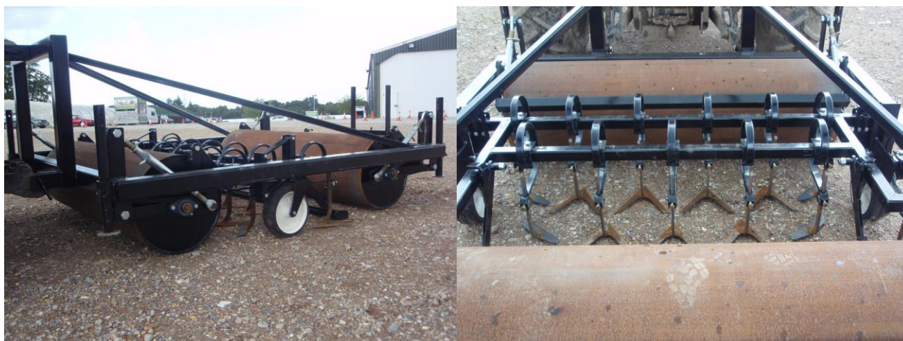
Figure 16. Twin roller false seedbed tiller. Design and photos copyright © Steam Weeding Ltd. 2015.
