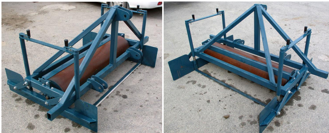
Figure 13. Roller undercutter false seedbed tiller, with front and rear undercutter bars plus side shields to retain bed sides. Design and photos copyright © Steam Weeding Ltd. 2015.
