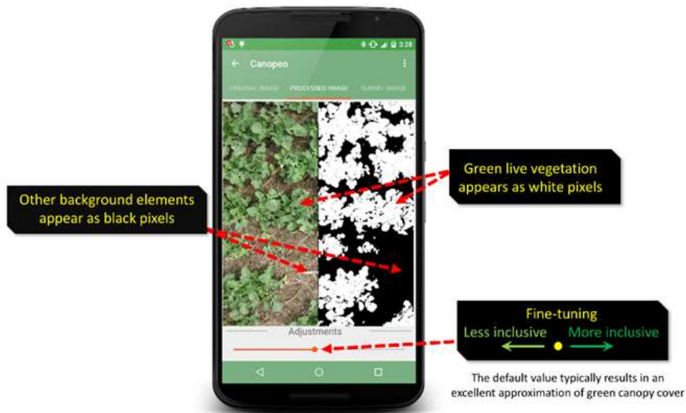
Figure 3: Canopeo app for recording ground cover
